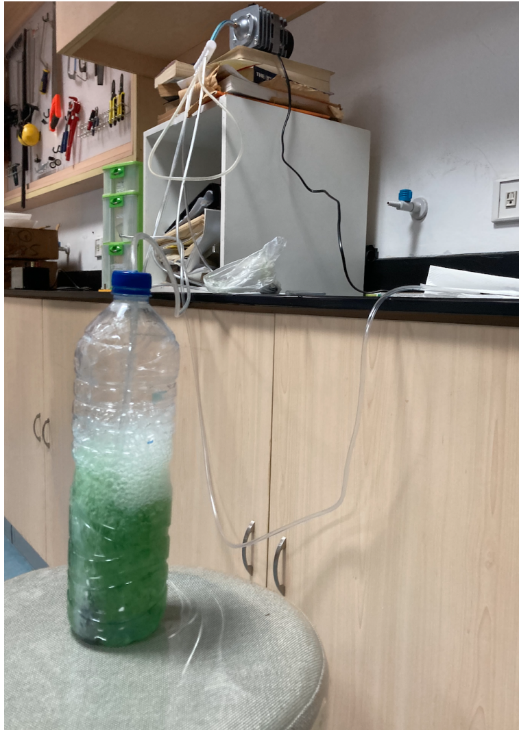
Figure 8: The testing in action. The air pump is situated above the box, which is piping air into the bottle of algae, distributed throughout the solution using an airstone. The air then flows out of the bottle, having been purified.
